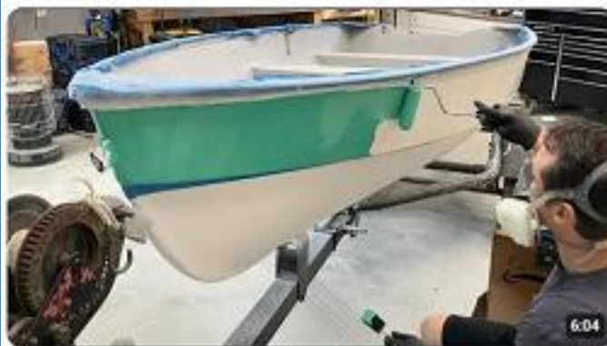
Pettit Paint - Rolling and Tipping EZ Poxo Boat Topside Paint is EZ!
